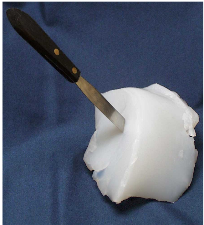
High Viscosity Silicone Polymer Mixed in the Ross Double Planetary Mixer equipped with HV Blades
