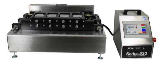
The Series 530 Horizontal Sealant Tester is designed to perform Aymar type tests at 1/8 inch per hour or variable speeds of 1/8 to 2 1/2 inches per minute according to ASTM C910, ASTM C736, ASTM C719, ASTM C1305, FEDERAL SS-S200, and FEDERAL TT-S230. We've improved upon our previous design with a touchscreen display, advanced controller options, and user friendly sample fixtures. When operating with an external freezer, users can now easily remove specimens without removing the entire machine.
